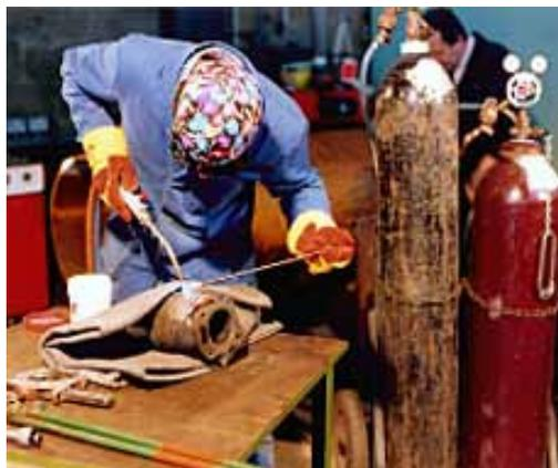
Figure 5. Basic Oxyfuel Welding Process.
