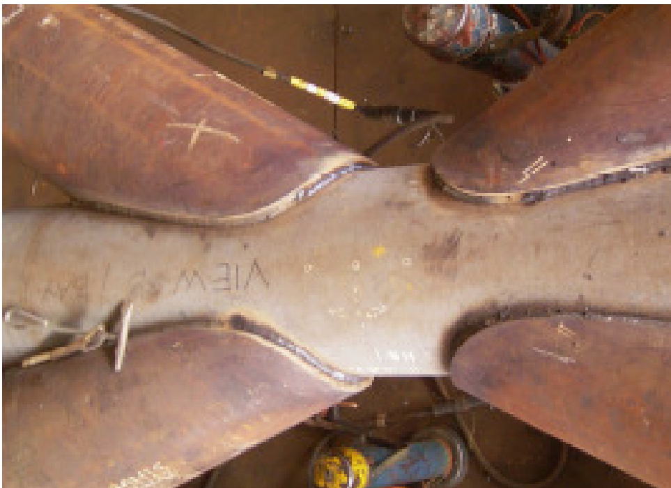
Figure 4. A typical node structure
