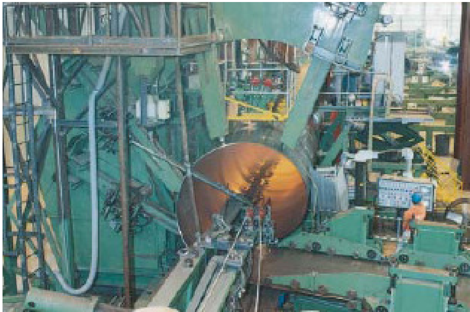
Figure 4. Typical SAW spiral welding station
